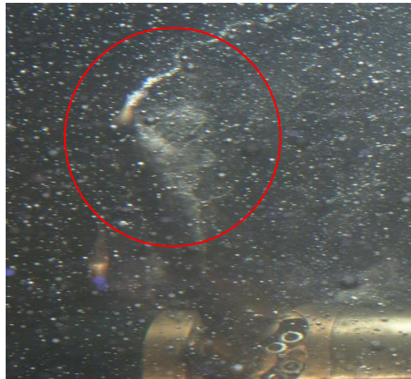
Fig. 7 Cavitation observed at 4.66 m/s current speed and \sigma=2.061
