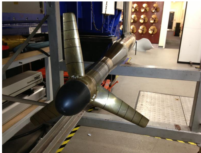
Fig. 3 Marine current turbine model mounted on Kempf &amp; Remmers type H33 dynamometer
