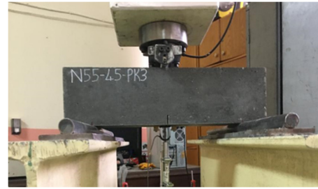
Fig. 2 Flexural test setup
