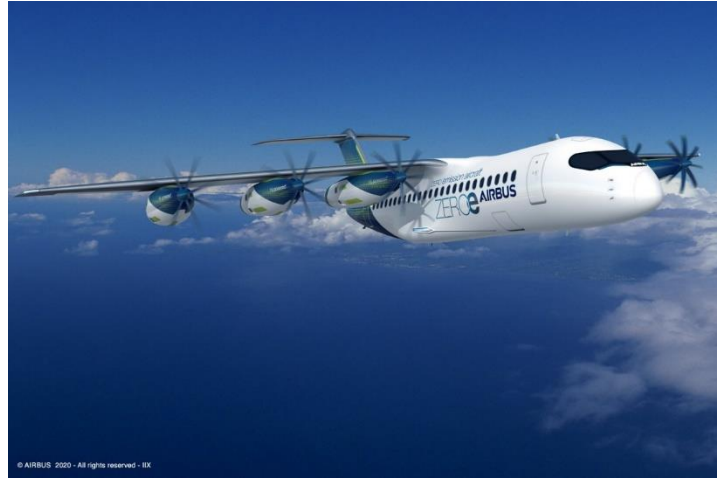
Fig. 14 Fuel cell “pods” propeller aircraft. Courtesy Airbus
