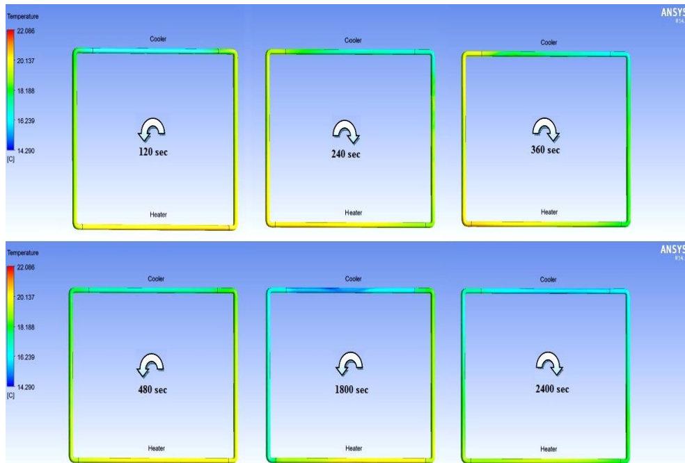
Fig. 17 Temperature distributions and fluid flow, power:100-watt
