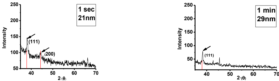
Fig. 2 XRD spectrum of Au NPs with different time of addition of reducing agent
