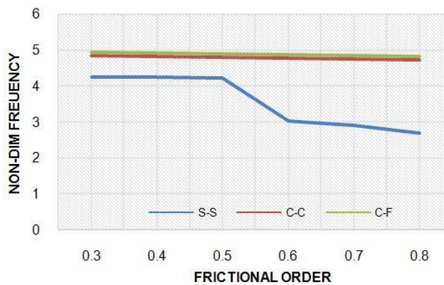
Fig. 10 Frictional order effect on vibration behavior of system under various boundary condition ( \mu = 1 \times 10^{-9} , L/h = 10 , g = 0.05 & K_G = 10 )
