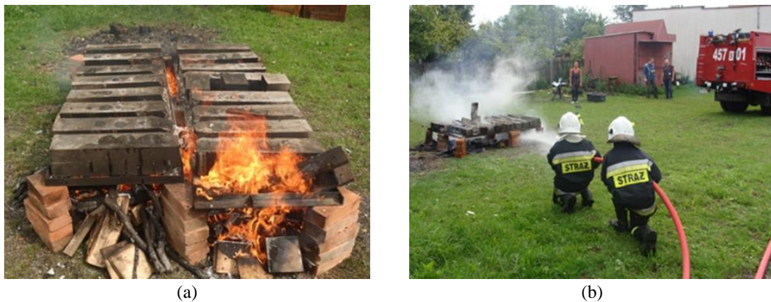
Fig. 3 Specimens during the fire test (a) and extinguishing the testing setup (b)
