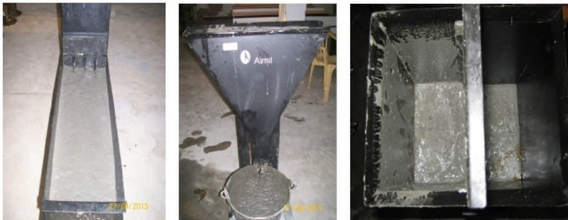
Fig. 5 (a) L-box test (b) V-funnel test (c) U-box test
