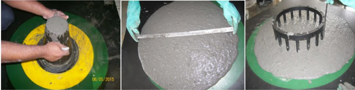
Fig. 4 (a) Slump flow test (b) T_{500} test (c) J-ring test
