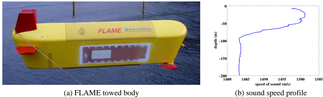
Fig. 1 (a) Picture of FLAME towed body with flat plate configuration (measurement area: white rectangle) during release from towing vessel RV ELISABETH MANN BORGESE, (b) sound velocity profile measured in Sognefjord, Norway, directly before the towing experiment
