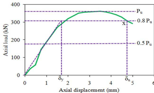
Fig. 10 Procedures for ductility calculation
