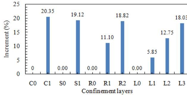
Fig. 7 Percent increment in ultimate load of various jacketed column with respect to confinement layers
