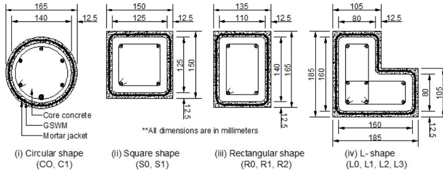
(a) Shapes section of test specimens
