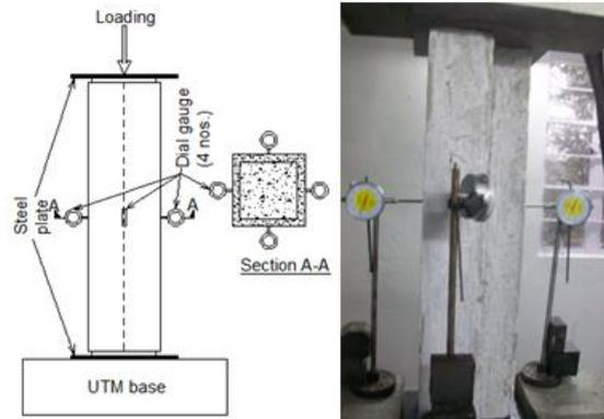
Fig. 5 Testing of specimens
