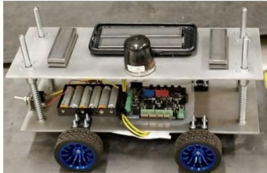
Fig. 2 Vehicle to induce vibration in the bridge
