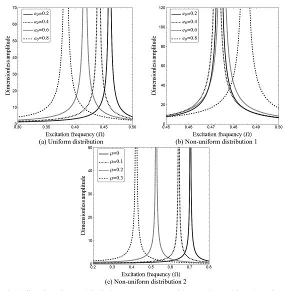
Fig. 6 Effect of pore factor and distribution on response curves of the nano-size metal foam plate (a/h=10,  $K_{w}=0$ ,  $K_{p}=0$ ,  $\mu=0.2$ ,  $\lambda=0.1$ )
