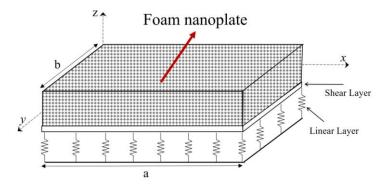
Fig. 2 Configuration of foam nanoplate under dynamical loading
