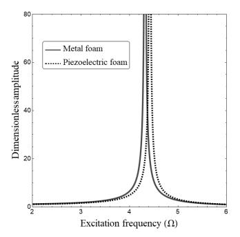
Fig. 5 Comparison between response curves of piezoelectric and metal foam nano-size plates (a/h=20,  $\mu=0.2$ ,  $\lambda=0$ ,  $e_0=0.2$ ,  $V_E=0$ )
