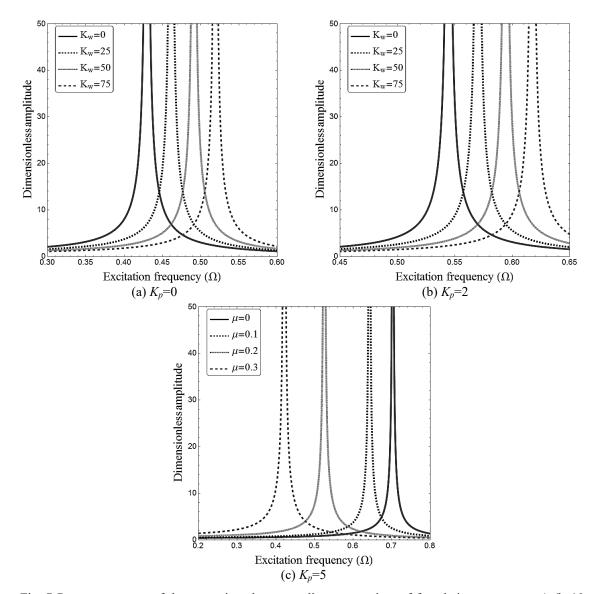
Fig. 7 Response curves of the nano-size plate according to a variety of foundation parameters (a/h=10,  $\mu=0.2$ ,  $e_0=0.5$ )
