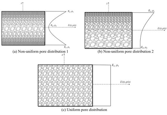
Fig. 1 Pore types along the thickness direction
