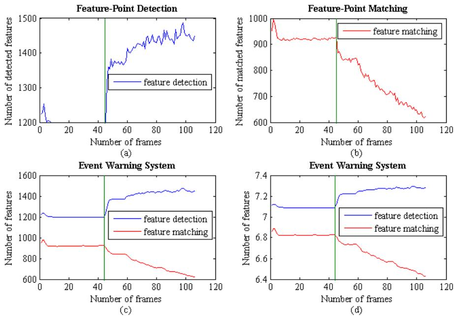
Fig. 3 The duration of the features in the debris flow sequence: (a) the number of detected features without smoothing, (b) the number of matched features without smoothing, (c) the combination of feature detection and feature matching with smoothing for the Hua-Shan area and (d) the combination of feature detection and feature matching with scaling using the log function for the Hua-Shan area
