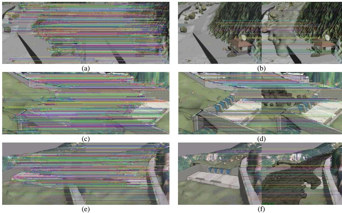
Fig. 1 The results of feature-point matching in the simulation environment.
