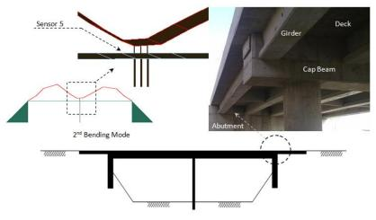
Fig. 8 Rigidity of the superstructure-pier connection
