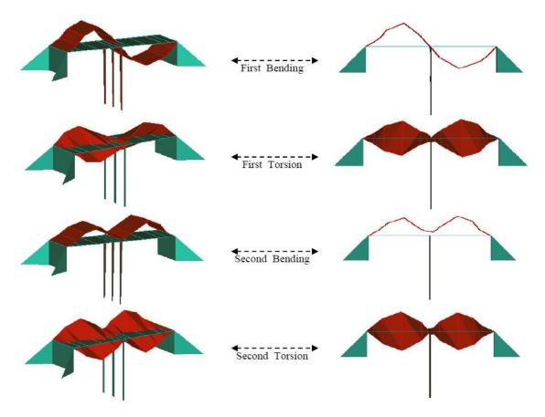
Fig. 6 Mode shapes identified from the first test carried out on the bridge
