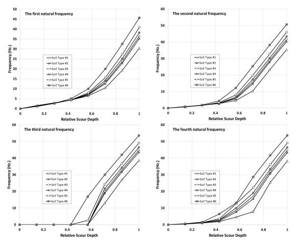
Fig. 14 Variation of the percent of reduction of the first four natural frequencies of the bridge with respect to the RSD for different sub-soils
