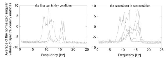
Fig. 5 The frequency domain decomposition plots derived from the tests on the bridge on two different condition of the riverbed
