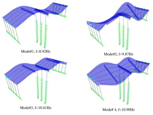
Fig. 10 Mode shapes obtained from the FE analysis of the bridge
