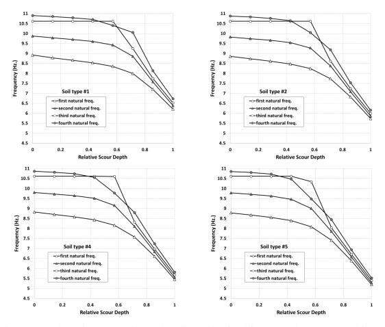
Fig. 15 Comparison of the natural frequencies of the bridge for different vibration modes and different sub-soils
