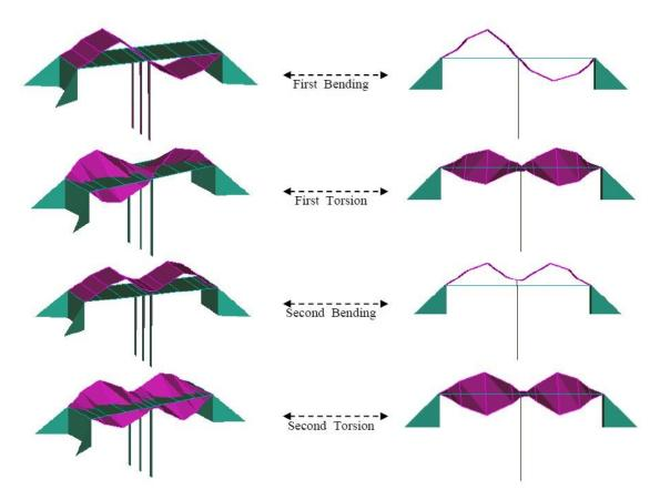
Fig. 7 Mode shapes identified from the second test carried out on the bridge
