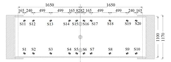
Fig. 3 The measurement grid of the test (dimensions are in cm)
