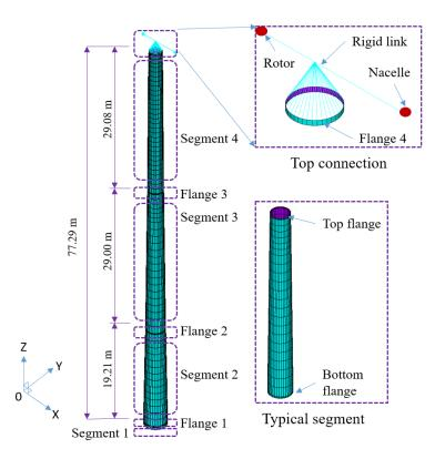
Fig. 6 Finite element modeling of the WTT
