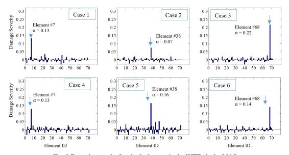
Fig. 9 Detection results for single damage in the WTT via the MAS
