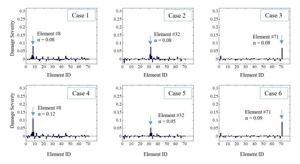
Fig. 8 Damage detection in the WTT model via the FAS
