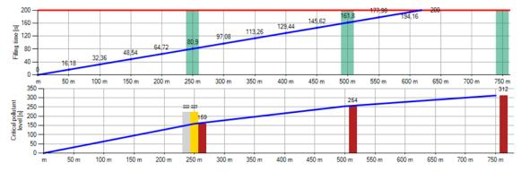
Fig. 4 (above) The tunnel filling time as result of traffic microsimulation model. Exits located every 250 m are highlighted in green. The time to the tunnel closure (200 s) is depicted as a red line); (below) Critical times [s] for CO propagation in grey and HCL propagation in yellow according to smoke propagation model and the custom physical model in brown
