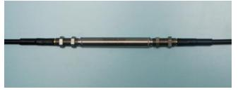
Fig. 7 FBG-based strain sensor
