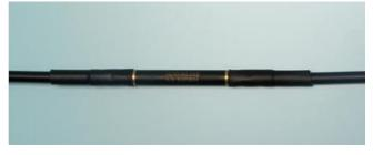
Fig. 8 FBG-based temperature sensor
