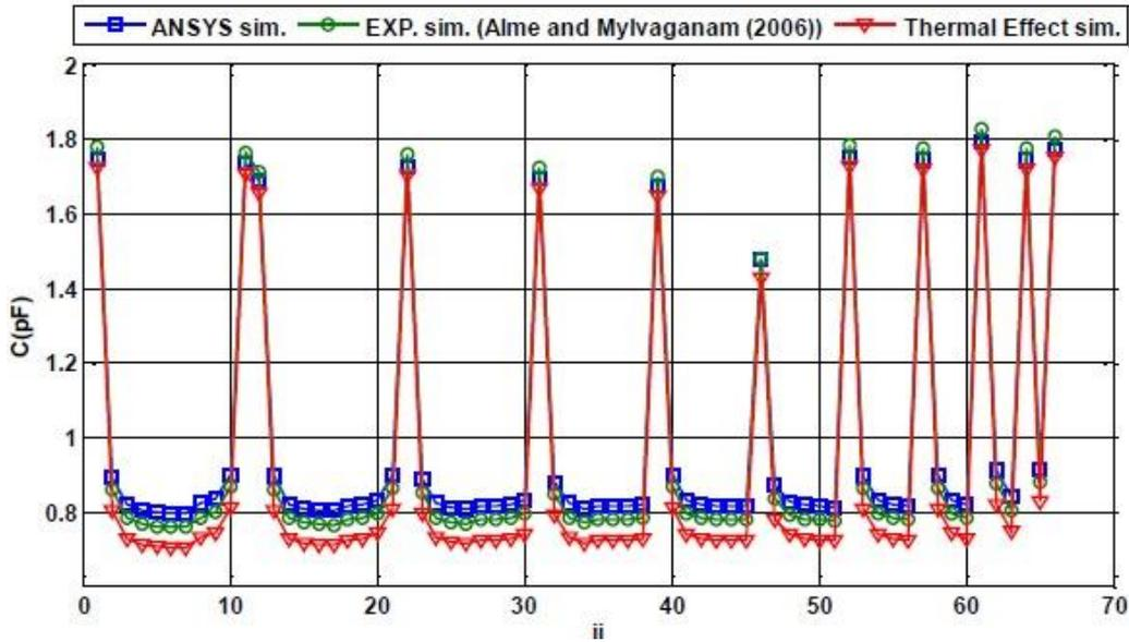
Fig. 6 Comparison of simulated capacitances from 2D ANSYS model for Air–Water two-phase flow between the 2D ANSYS model and experimental model at room temperature and with thermal effect.
