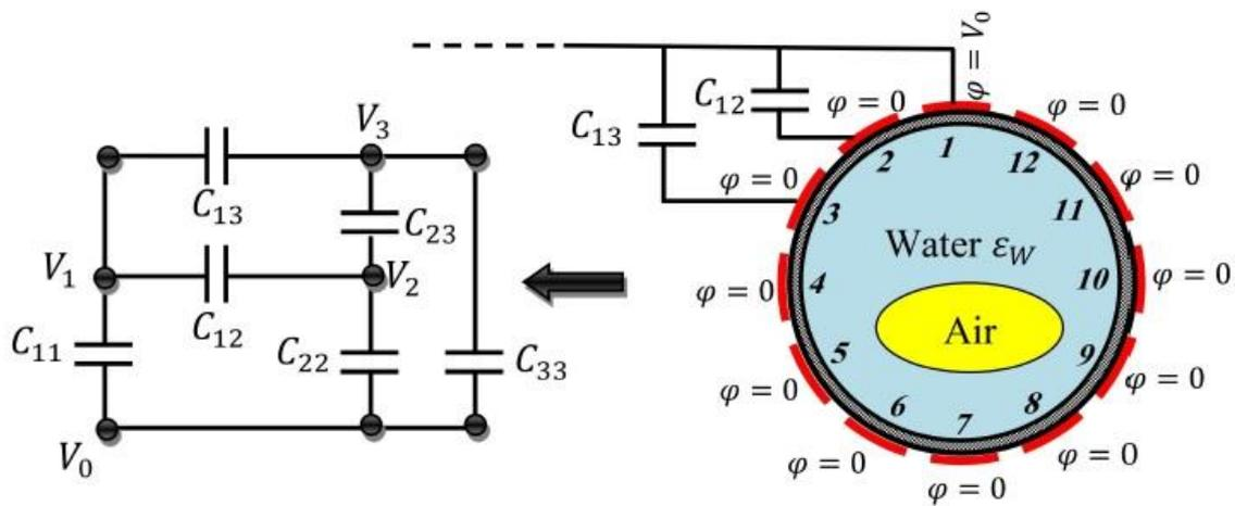
Fig. 3 Schematic representation of the measurement principle of an ECS
