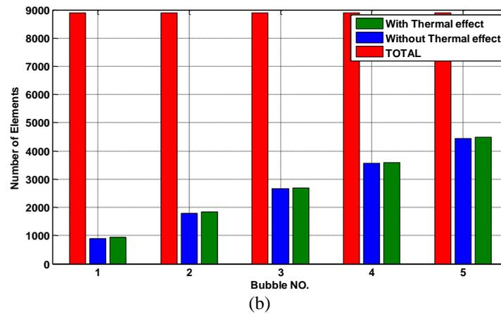
Fig. 8 (a) The water distribution across pipe at room temperature and with thermal effect and (b) The Air distribution across pipe at room temperature and with thermal effect
