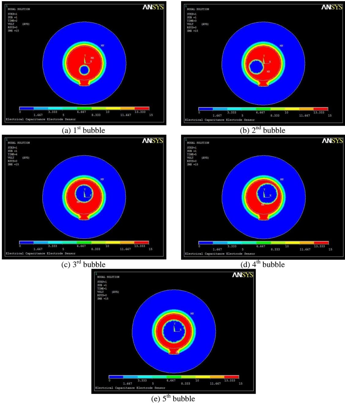
Fig. 5 node potential equivalent of Air–Water two-phase flow measurements from ANSYS 2D model
