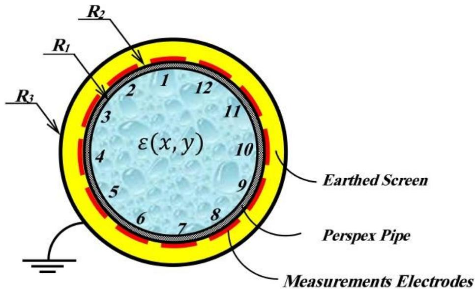
Fig. 2 Cross section sketch of 12-electrode ECS
