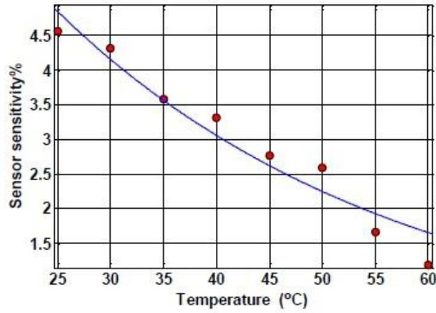
Fig. 7 Capacitance sensor sensitivity versus Temperature (°C)
