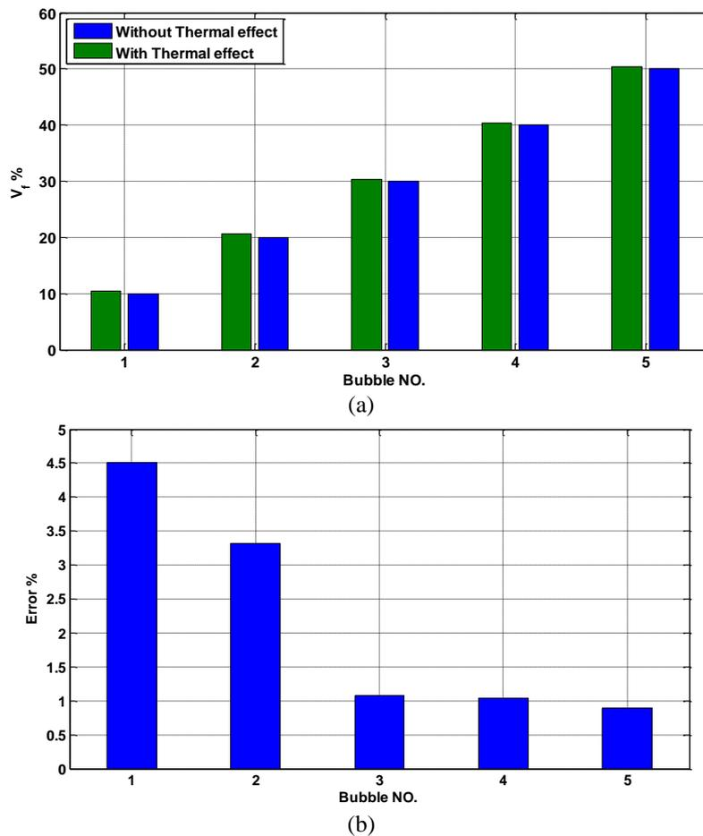
Fig. 9 (a) The void fraction  $V_f\%$  distribution at room temperature and with thermal effect and (b) The Air void fraction distribution error due to thermal effect
