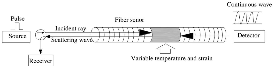
Fig. 1 Sensing principle of BOTDA
