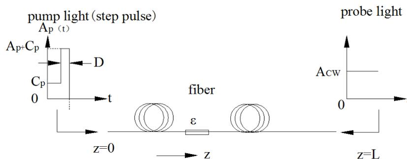
Fig. 2 Monitoring principle of PPP-BOTDA technology
