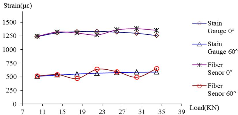
Fig. 6 Results of fiber sensor and strain gauge under the bending and stretching load
