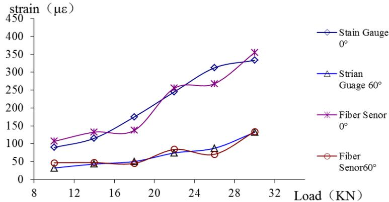
Fig. 5 Results for fiber sensor and strain gauge
