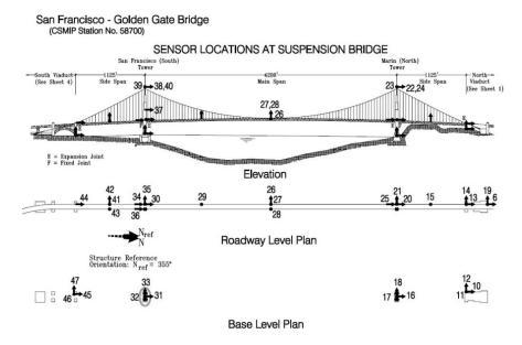
Fig. 5 Golden Gate bridge instrumentation (http://www.strongmotioncenter.org)
