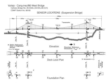
Fig. 8 Alfred Zampa bridge instrumentation (http://www.strongmotioncenter.org)
