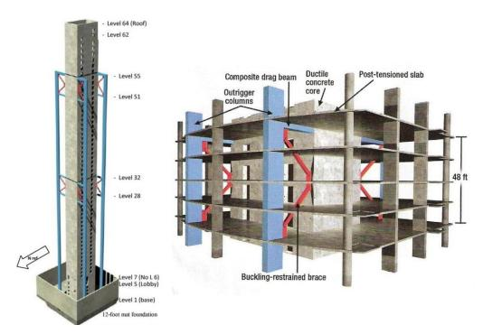
Fig. 3 One Rincon Hill Tower structural system (Huang et al. 2012)
