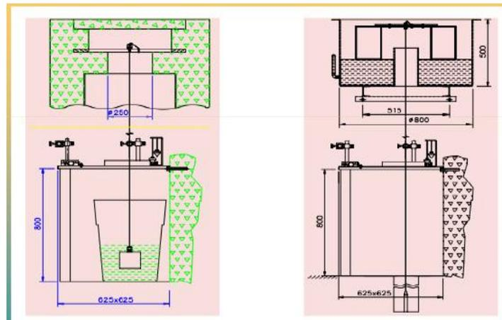
Fig. 6 Installation diagram of Normal and inverted plumb line
