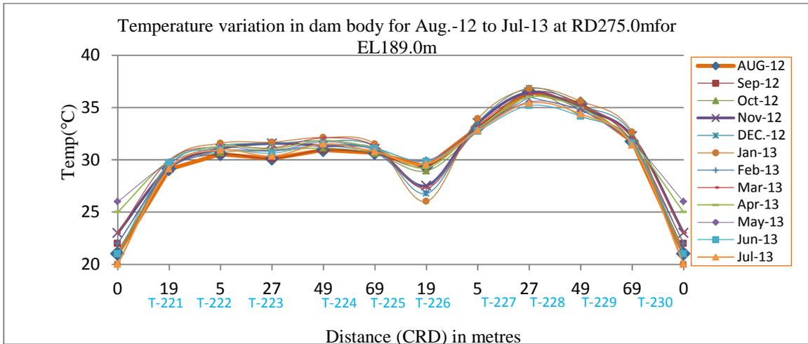
Fig. 12 Variation in temperature in horizontal direction within dam body during various months
