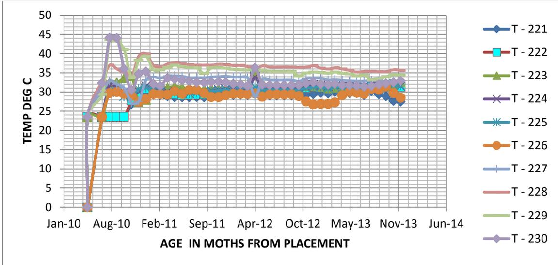
Fig. 11 Temperature -time history across RCC layer as recorded by thermocouples
