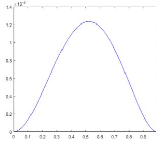
Fig. 4 The solution curve in the case of a fixed supported beam along inhomogeneity  $f(\zeta) = \sin(\zeta)$
