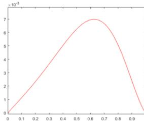
Fig. 9 The solution curve in the case of a simply supported beam along inhomogeneity  $f(\zeta) = \zeta^2$
