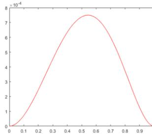
Fig. 3 The solution curve in the case of a fixed supported beam along inhomogeneity  $f(\zeta) = \zeta^2$
