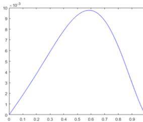
Fig. 10 The solution curve in the case of a simply supported beam along inhomogeneity  $f(\zeta) = \sin(\zeta)$
