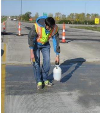
Fig. 19 Crack survey using wet test method (water wetting of concrete surface)
