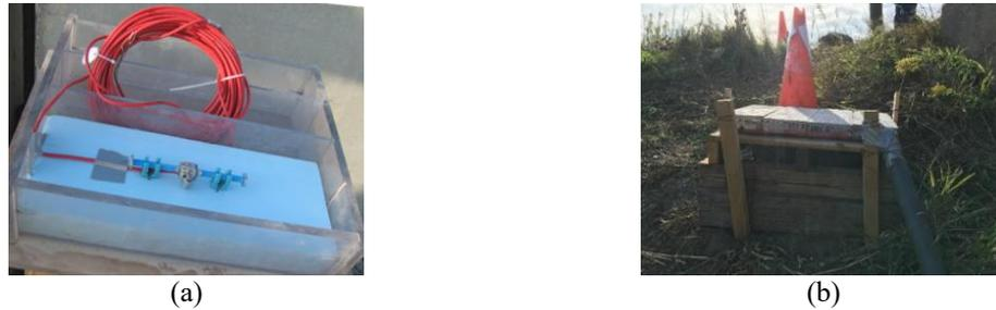
Fig. 10 (a) Mini slab mold and strain gauge location and (b) Mini slabs on the field site
