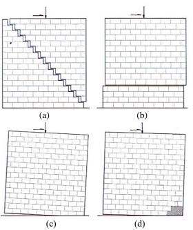
Fig. 5 In-plane failure modes of a laterally loaded URM wall: (a) shear failure, (b) sliding failure, (c) rocking failure and (d) toe crushing. (ElGawady *et al.* 2006)
