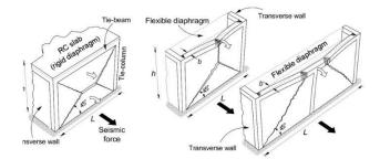
Fig. 6 The out-of-Plane failure mechanism of masonry wall (Source: http://achyutpaudel.com.np/)
