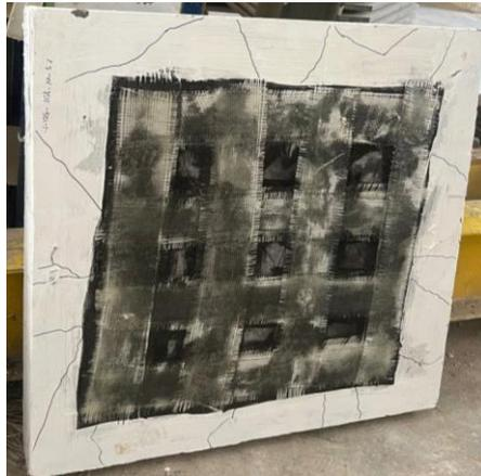
Fig. 29 Failure pattern of (V-125-2GF-1%-M)
