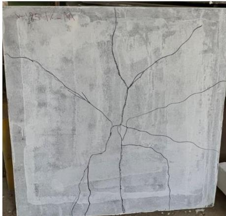
Fig. 28 Failure pattern of (V-125-1%-M)
