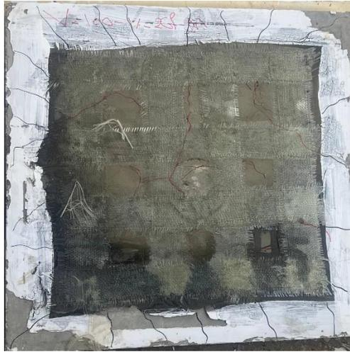
Fig. 30 Failure pattern of (V-100-2GF-1%-M)
