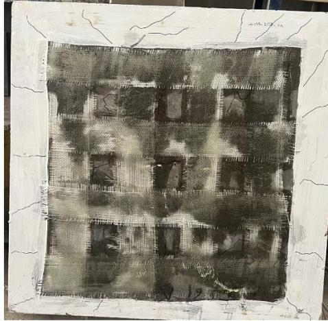
Fig. 27 Failure pattern of (V-125-2GF-M)
