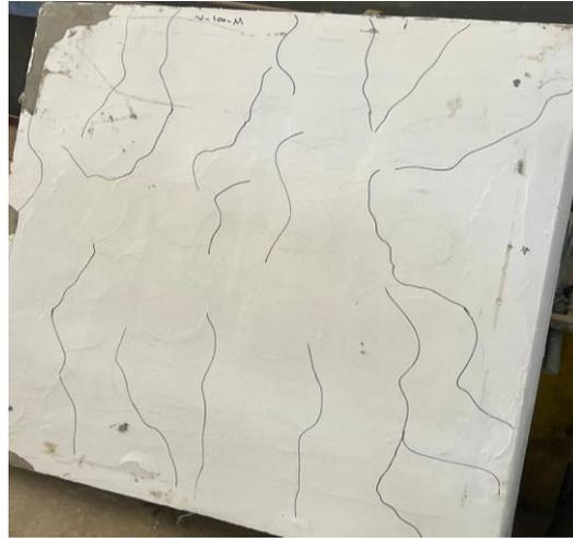
Fig. 25 Failure pattern of (V-100-M)
