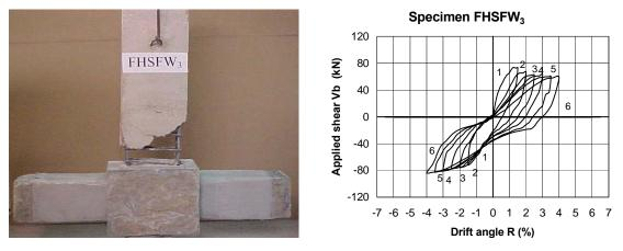
Fig. 6 Plots of applied shear versus drift angle and failure mode of the strengthened subassemblage  $FHSFW_3$
