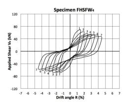
Fig. 7 Plots of applied shear versus drift angle and failure mode of the strengthened subassemblage  $FHSFW_4$
