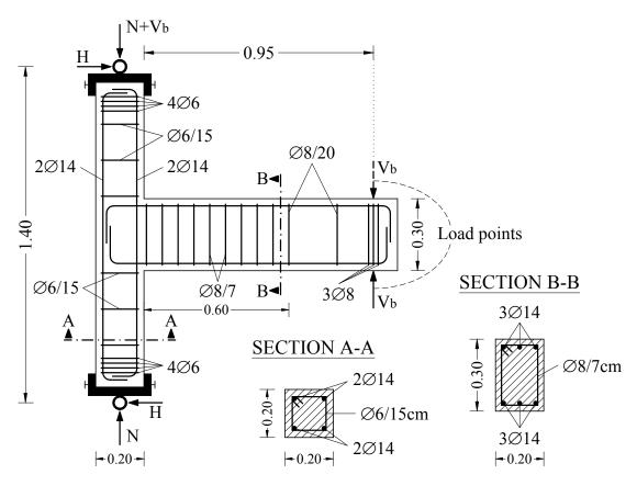
Fig. 1 Dimensions and cross-sectional details of original subassemblages O<sub>3</sub>, W<sub>2</sub>, W<sub>3</sub>, M<sub>1</sub>, and M<sub>3</sub>
