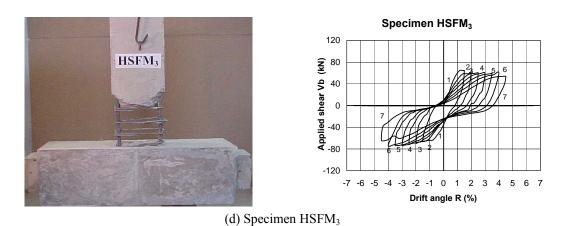
Fig. 4 Plots of applied shear versus drift angle and failure mode of the strengthened subassemblages  $SO_3$ ,  $FW_2$ ,  $HSFM_1$  and  $HSFM_3$
