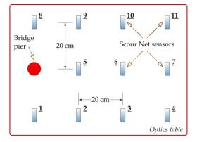
Fig. 7 The layout of the 11 distributed Scour Net sensors mounted on top of an optics table is shown. Sensor IDs are labeled in bold and underlined
