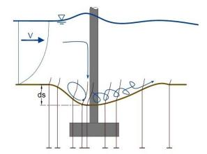
Fig. 1 The schematic illustrates the operating principle of the distributed Scour Net monitoring system. Buried cantilevered piezoelectric strips become exposed due to scour hole evolution
