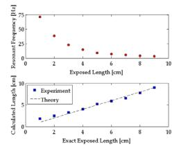
Fig. 4 (Top) The resonant frequencies for the nine different exposed lengths were extracted from the power spectral density plots. Resonant frequencies decreased with increasing scour depths. (Bottom) The calculated scour depths were also compared to theoretical results (i.e., direct measurements)
