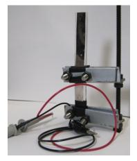
Fig. 2 A Scour Net sensor was configured to form a vertical cantilevered beam and was attached on a customized mount for experimental testing. The exposed length was adjusted by sliding the top security mount up or down (i.e., for simulating scour)
