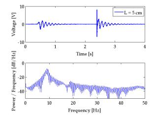
Fig. 3 A Scour Net sensor with a 5 cm exposed length was tested in air. (Top) The voltage time history responses showed the free vibration responses of the Piezo Film-PDMS sensor. (Bottom) The corresponding power spectral density function showed that the resonant frequency was 9.0 Hz
