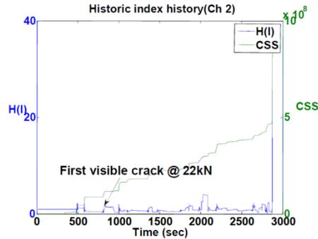
Fig. 10 Beam SD1: H(I)-CSS plot for R151 sensor located close to end of FRP strip
