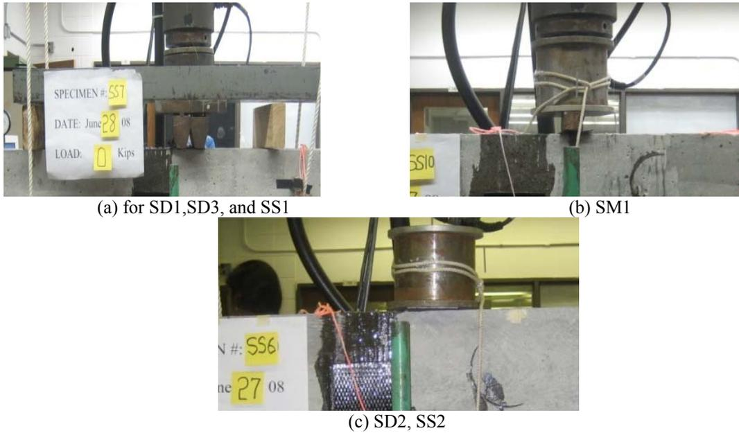
Fig. 3 Load transfer mechanisms
