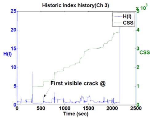
Fig. 25 Beam SM1: H(I)-CSS plot for R15I sensor
