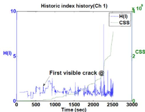
Fig. 15 Beam SS1: H(I)-CSS plot for R6I sensor
