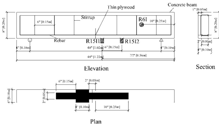
Fig. 2 Beam specimen details
