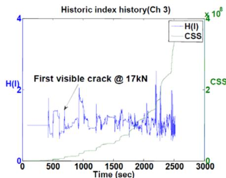
Fig. 16 Beam SS1: H(I)-CSS plot for R15I sensor
