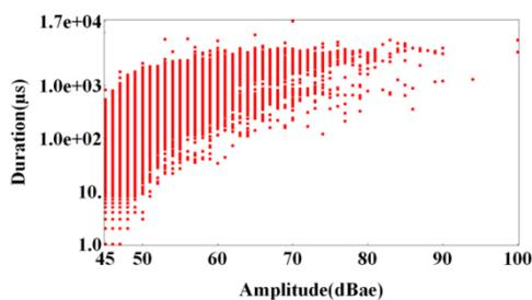
Fig. 14 Beam SS1: Amplitude vs Duration
