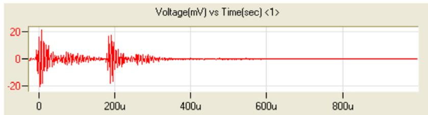
Fig. 8 Double hit AE signal waveform
