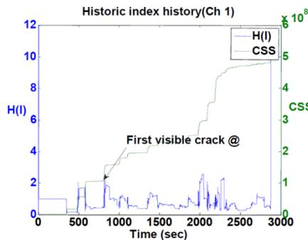
Fig. 9 Beam SD1: H(I)-CSS plot for R15I sensor located close to center of beam
