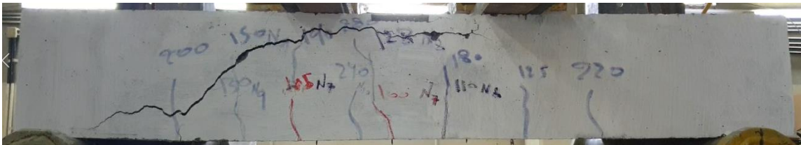
Fig. 11 Crack pattern at ultimate load for HCCS (100 mm) (Slab-9) repeated test
