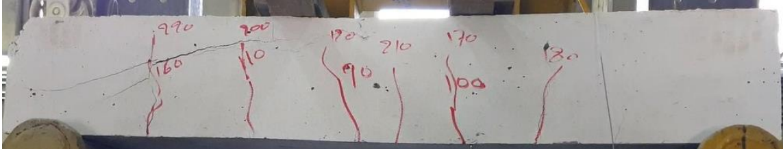
Fig. 14 Crack pattern at ultimate load for HSCS dimensions (57x57) mm (Slab-5) monotonic test
