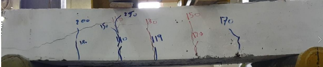
Fig. 9 Crack pattern at ultimate load for HCCS (50 mm One Core) (Slab-8) repeated test
