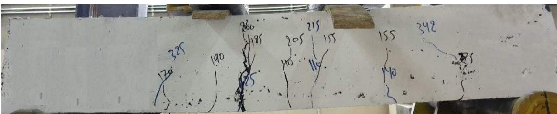
Fig. 17 Crack pattern at ultimate load for HCCS (100 mm) with S. F (Slab-12) repeated test
