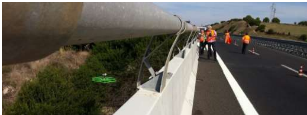
Fig. 1 Unmanned Aerial Vehicle (UAV) for visual inspection (Aibotix GmbH, 2014)
