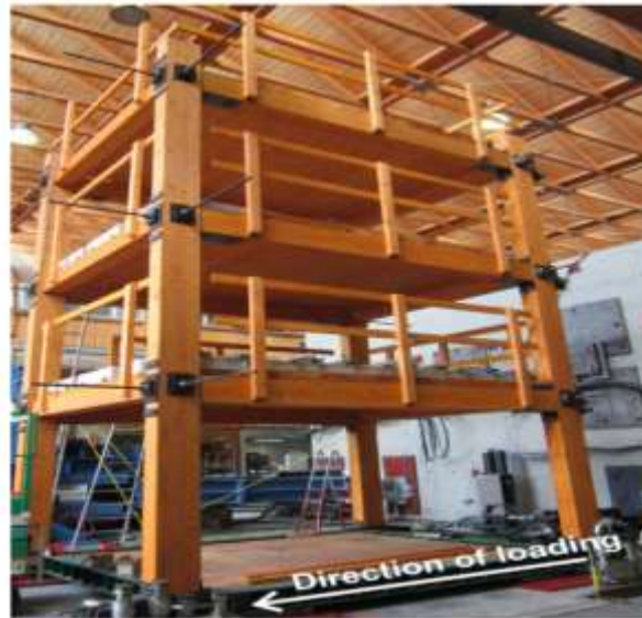
Fig. 1 Experimental post-tension frame constructed in UNIBAS laboratory, Italy, in collaboration with the University of Canterbury in Christchurch, New Zealand (Ponzo et al. 2012)
