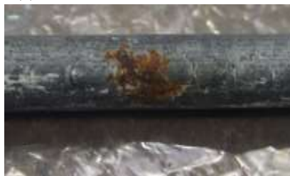
(b) Attack on steel bar surface
