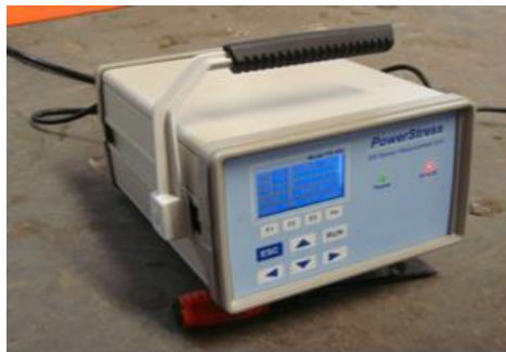
Fig. 5 PS-500 data acquisition instrument (magnetoelastic instrument)
