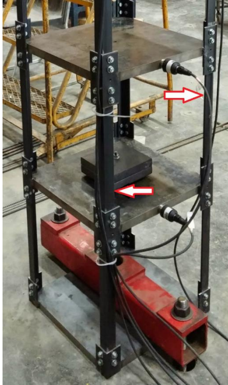
Fig. 3 Damage Pattern 1: Replacing two thinner columns between the first and second floors
