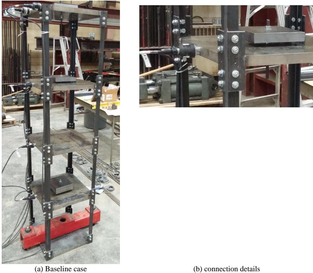
Fig. 1 The experimental structure
