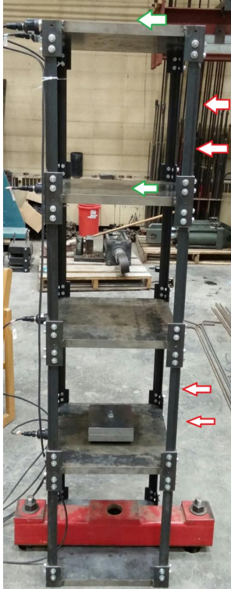
Fig. 8 Damage Pattern 6: Removing one plate at the third floor +DP5
