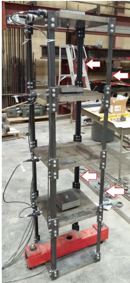
Fig. 5 Damage Pattern 3: Replacing two thinner columns between the first and second floors; the third and fourth floors
