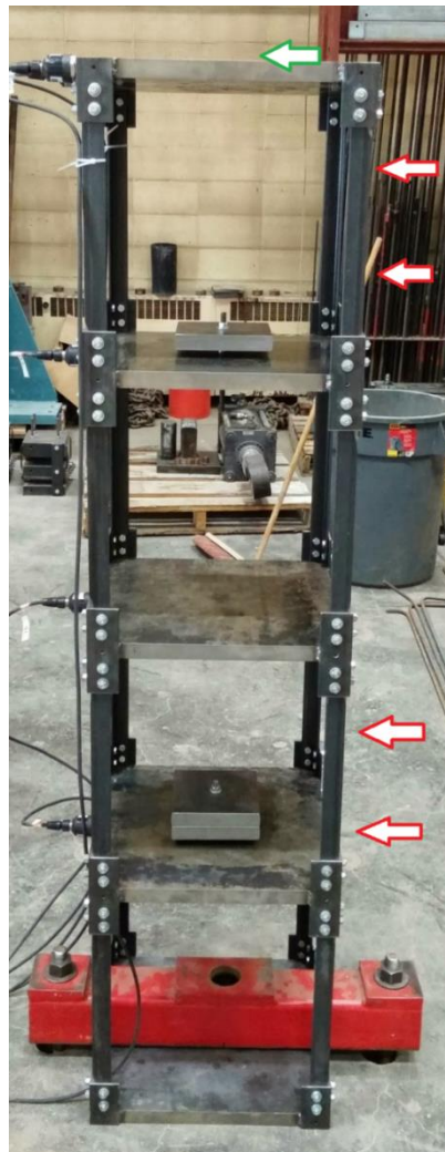
Fig. 7 Damage Pattern 5: Removing one plate at the fourth floor +DP3
