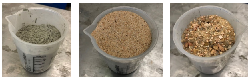
Fig. 6 Materials for experiment concrete casting (left: cement, middle: sand, right: sand and coarse aggregate)
