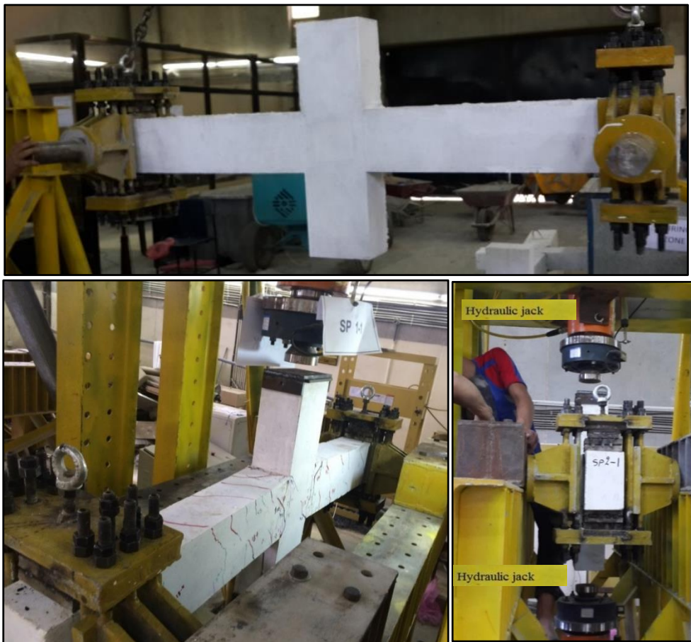
Fig. 8 The supporting system, hydraulic jacks, and the test setup
