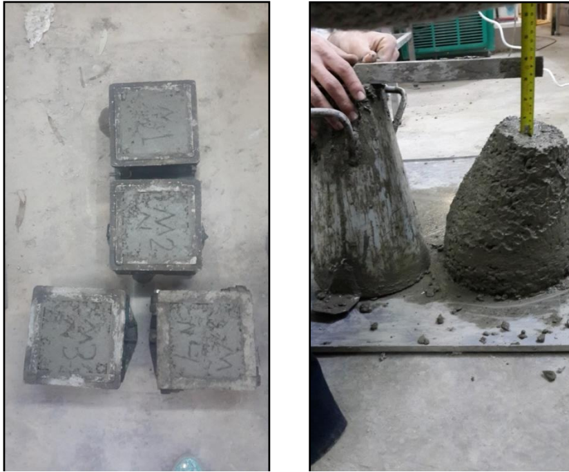
Fig. 7 Sampling and testing of fresh concrete
