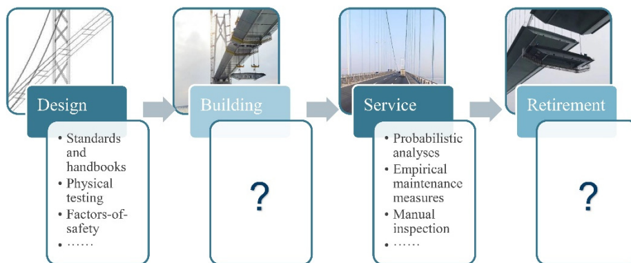
Fig. 1 Current fatigue management during steel bridge lifecycle
