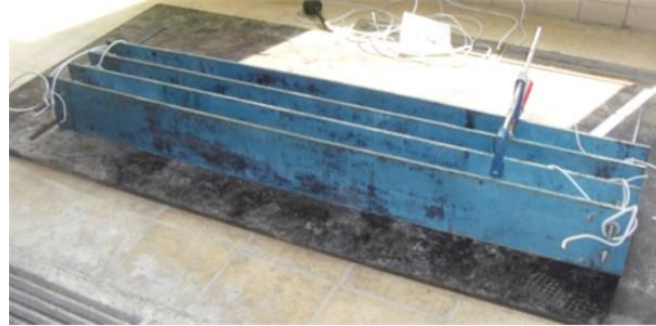
(a) The molds used to cast the model piles
