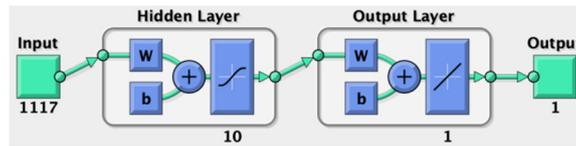
Fig. 4 Neural network of the first NN model (The number of hidden layers = 10)
