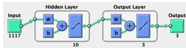
Fig. 8 Neural network of the third NN model (the number of hidden nodes = 10)
