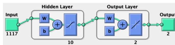
Fig. 6 Neural network of the second NN model (the number of hidden nodes = 10)
