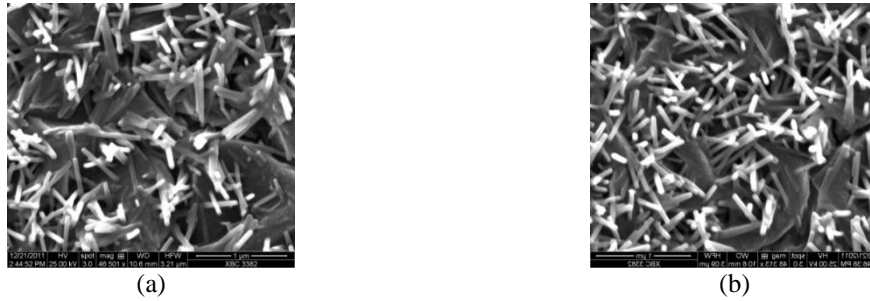
Fig. 4 SEM micrographs of the two types of samples are shown. (a) A view of a ZnO-PDMS sample, exhibiting fairly dense growth, (b) A view of a ZnO-PDMS/rGO sample exhibiting similarly dense growth. Note: the small gaps between the nanorods in both the samples
