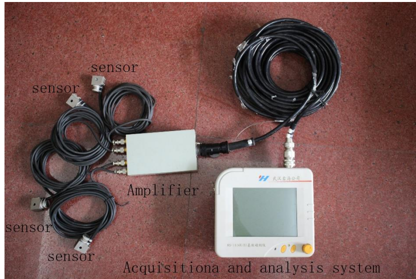
Fig. 10 Multi-channel reflected wave pick-up device
