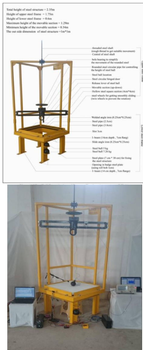
Fig. 1 Impact testing machine with sensors
