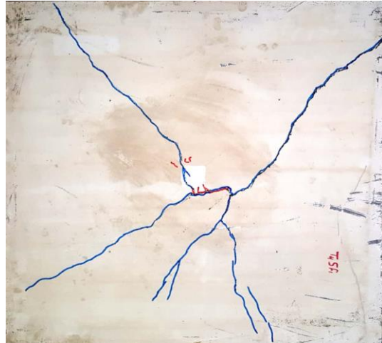
Fig. 8 Dynamic-static crack pattern of the slab T4SF1
