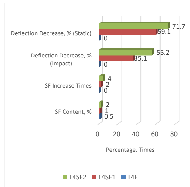
Fig. 13 Effect of steel fiber content increase times on the dynamic and static deflection of HP concrete slabs
