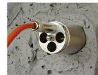
(b) Reference head, transducer and electrical readout device (MC7)
