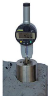
(a) Reference head (collar) and mechanical readout device (ERDM50+)
