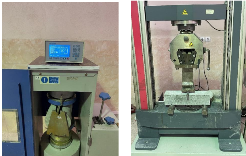
Fig. 6 (a) ADR-Touch device for compressive and tensile strength tests and (b) universal device for bending strength tests
