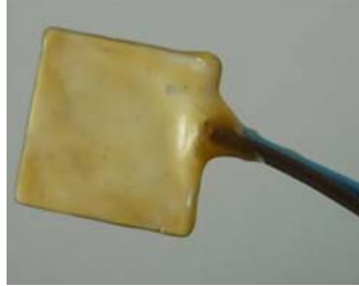
Fig. 8 the waterproof layer by epoxy resin (Zhao 2008)
