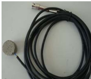
Fig. 6 Embedded cement based PZT sensor (Zhao 2008)
