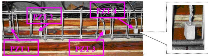
(a) Arrange of PZT sensors in reinforced concrete beam
