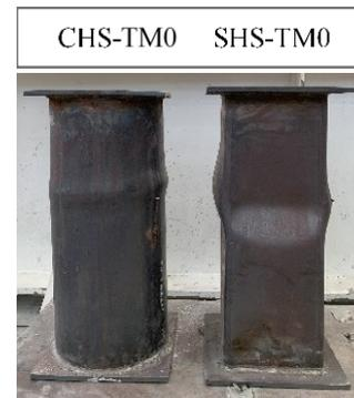
Fig. 12 Hollow columns after the tests
