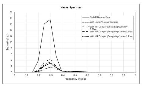
Fig. 11 Semisubmersible heave spectra (with and without damper)
