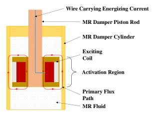
Fig. 1 Schematic and configuration of an MR damper
