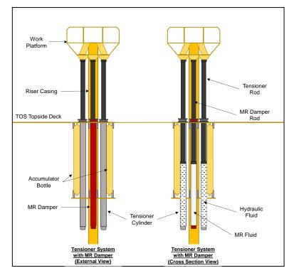
Fig. 4 Riser system top elevation view with tensioner and damper
