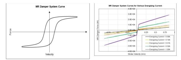
Fig. 2 Generic MR damper system curve (left) and scaled MR damper system damping curve for various energizing current (right)
