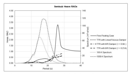
Fig. 7 Input wave spectra and heave RAOs for free-floating and with TTR+dampers cases
