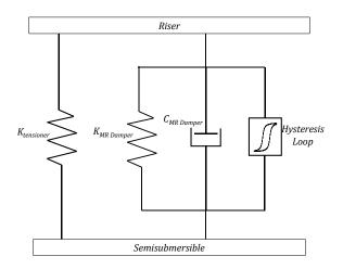
Fig. 5 A Free-body diagram of MR damper in riser tensioner system
