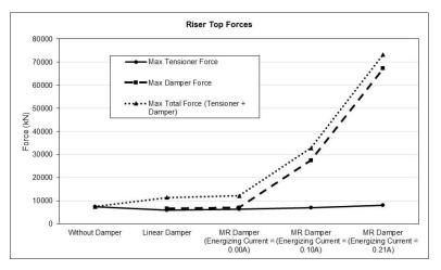
Fig. 13 Riser-top forces (Tensioner w/wo dampers)
