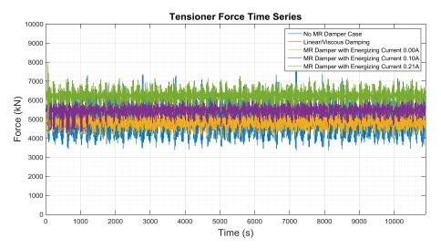
Incorporating magneto-Rheological damper into riser tensioner system to restrict riser stroke ... 115
