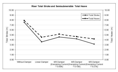
Fig. 12 Riser total stroke (TTR2) and semisubmersible total heave
