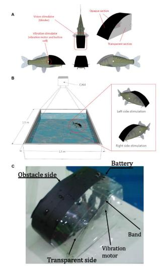
Fig. 2 Schematic of the experimental device and settings for the turning behavior test. (a) The stimulation device used to induce carp (C. carpio) obstacle avoidance behavior. The device consists of a blinder, vibration motor, and button cell. (b) Experimental setup for the turning behavior test. The water depth was 0.6 m. (c) Stimulation device
