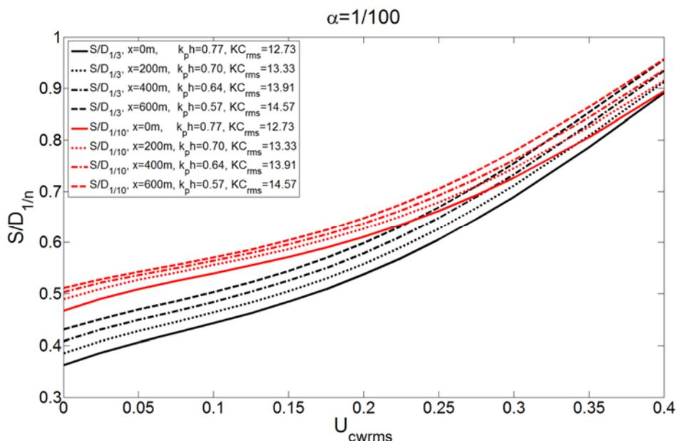
Fig. 14  $S/D_{1/3}$  and  $S/D_{1/10}$  for  $n=(3, 10)$  versus  $U_{cwrms}$  at four locations for slope  $\alpha=1/100$
