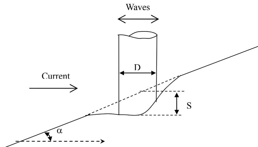
Fig. 2 Definition sketch of the scour depth ( $S$ ) around a circular vertical pile with diameter ( $D$ ) on a mild slope ( $\alpha$ )
