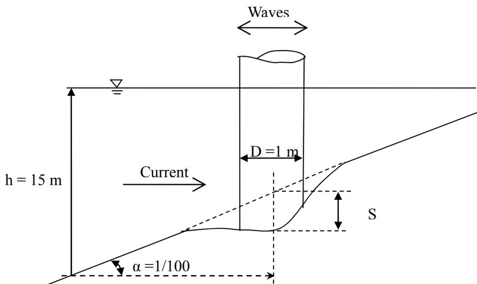
Fig. 3 Definition sketch of the seabed conditions with  $\alpha = 1/100$
