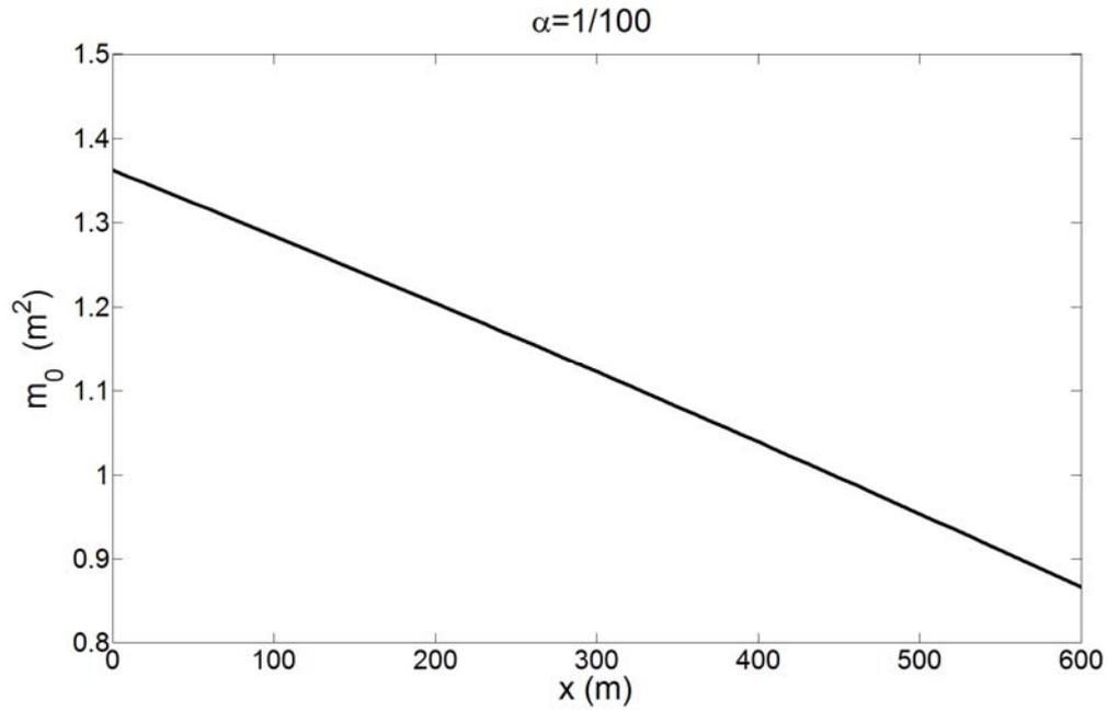
Fig. 5 Zeroth wave spectral moment  $m_0$  versus  $x$  in finite water depth for slope  $\alpha = 1/100$
