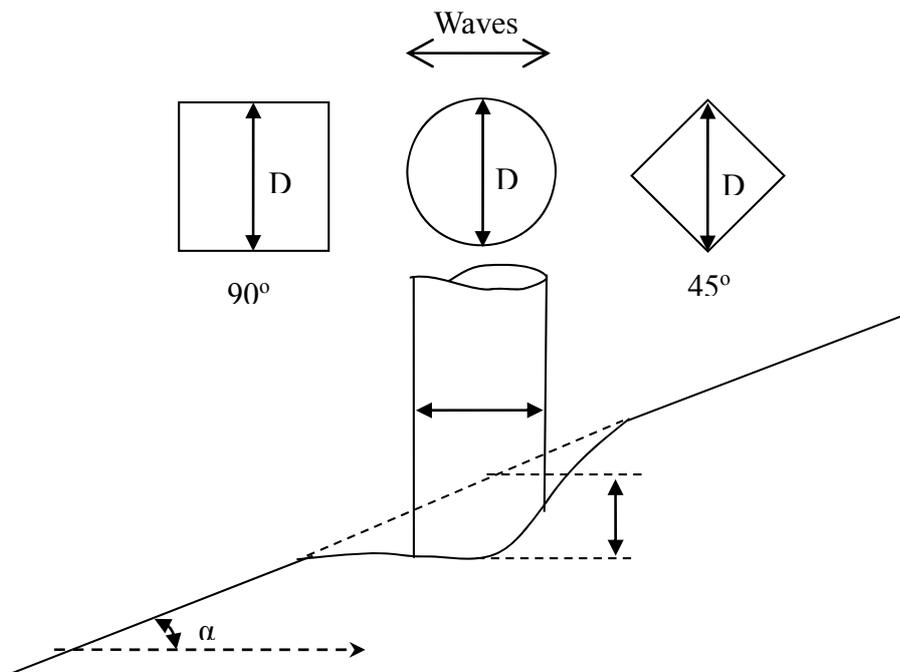
Fig. 17 Definition sketch of the scour depth ( $S$ ) around vertical piles with diameter ( $D$ ) and different shapes on a mild slope ( $\alpha$ )
