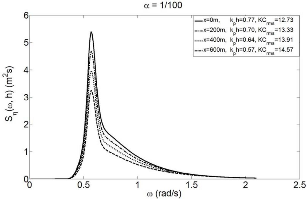
Fig. 4 The transitional wave spectra in finite water depth  $S_{\eta}(\omega, h)$  versus  $\omega$  at four locations for slope  $\alpha = 1/100$
