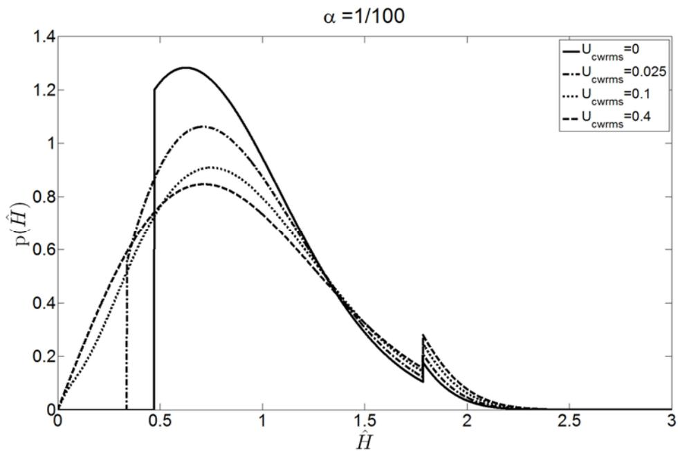
Fig. 13 Truncated pdf of  $\hat{H}$  for four different values of  $U_{cw rms}$  at location 1 ( $x = 0, h = 15$  m) for slope  $\alpha = 1/100$
