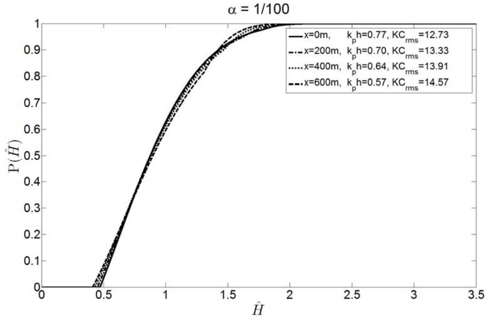
Fig. 8 Truncated *cdf* of  $\hat{H}$  at four locations for slope  $\alpha = 1/100$
