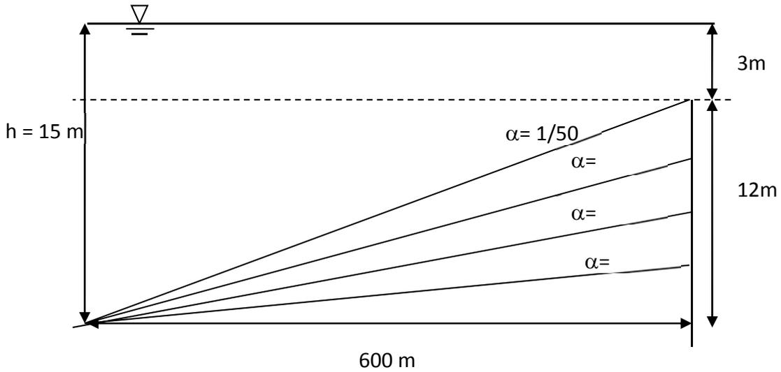
Fig. 10 Sketch of the seabed conditions for four slopes  $\alpha = (1/50, 1/100, 1/150, 1/250)$ . The total horizontal length of the sloping bed is 600 m, and the water depth at the seaward location is 15 m
