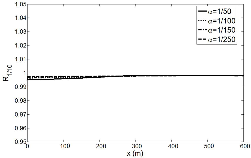
Fig. 15 Random waves alone: The stochastic to approximate method ratio  $R_{1/10}$  (i.e.,  $n = 10$ ) versus  $x$  for four slopes  $\alpha = ( 1/50, 1/100, 1/150, 1/250)$
