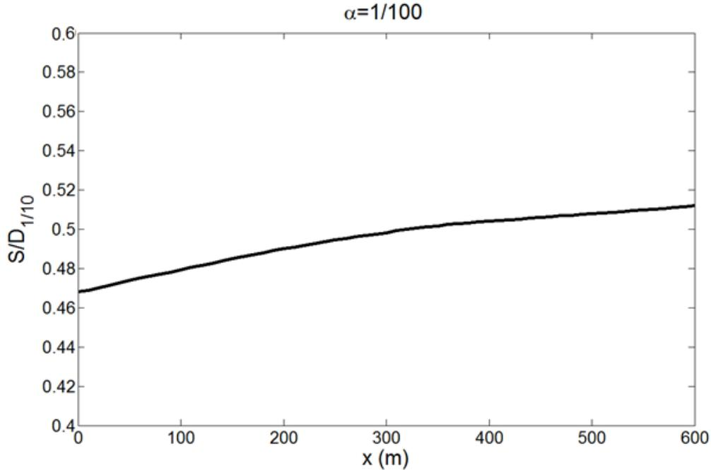
Fig. 9  $S/D_{1/10}$  versus  $x$  in finite water depth for slope  $\alpha = 1/100$
