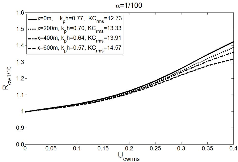
Fig. 16 Random waves plus current: The stochastic to approximate method ratio  $R_{cw1/10}$  (i.e.,  $n = 10$ ) versus  $U_{cwrms}$  at four locations for slope  $\alpha = 1/100$
