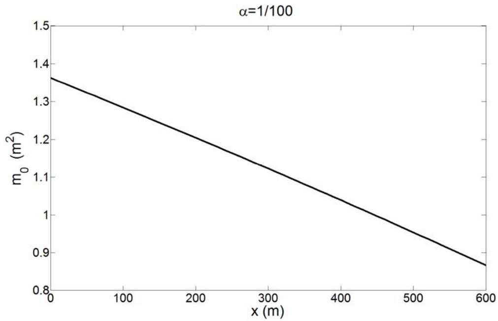
Fig. 5 Zeroth wave spectral moment  $m_0$  versus  $x$  in finite water depth for slope  $\alpha = 1/100$
