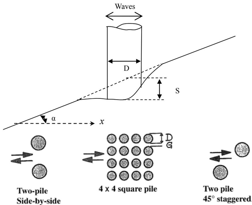
Fig. 18 Definition sketch of pile arrangements for  $G/D = 0.4$  and scour-depth ( $S$ ) around vertical pile on a mild slope ( $\alpha$ ) (reproduced from Sumer and Fredsøe (1998))
