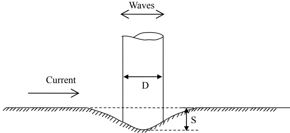
Fig. 1 Definition sketch of the scour depth ( $S$ ) around a circular vertical pile with diameter ( $D$ ) on a horizontal bed
