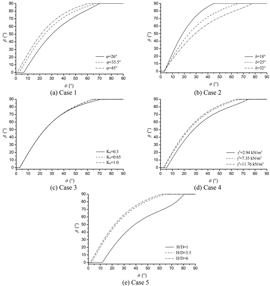
Fig. 3 Effects of different parameters on the failure direction of suction anchors
