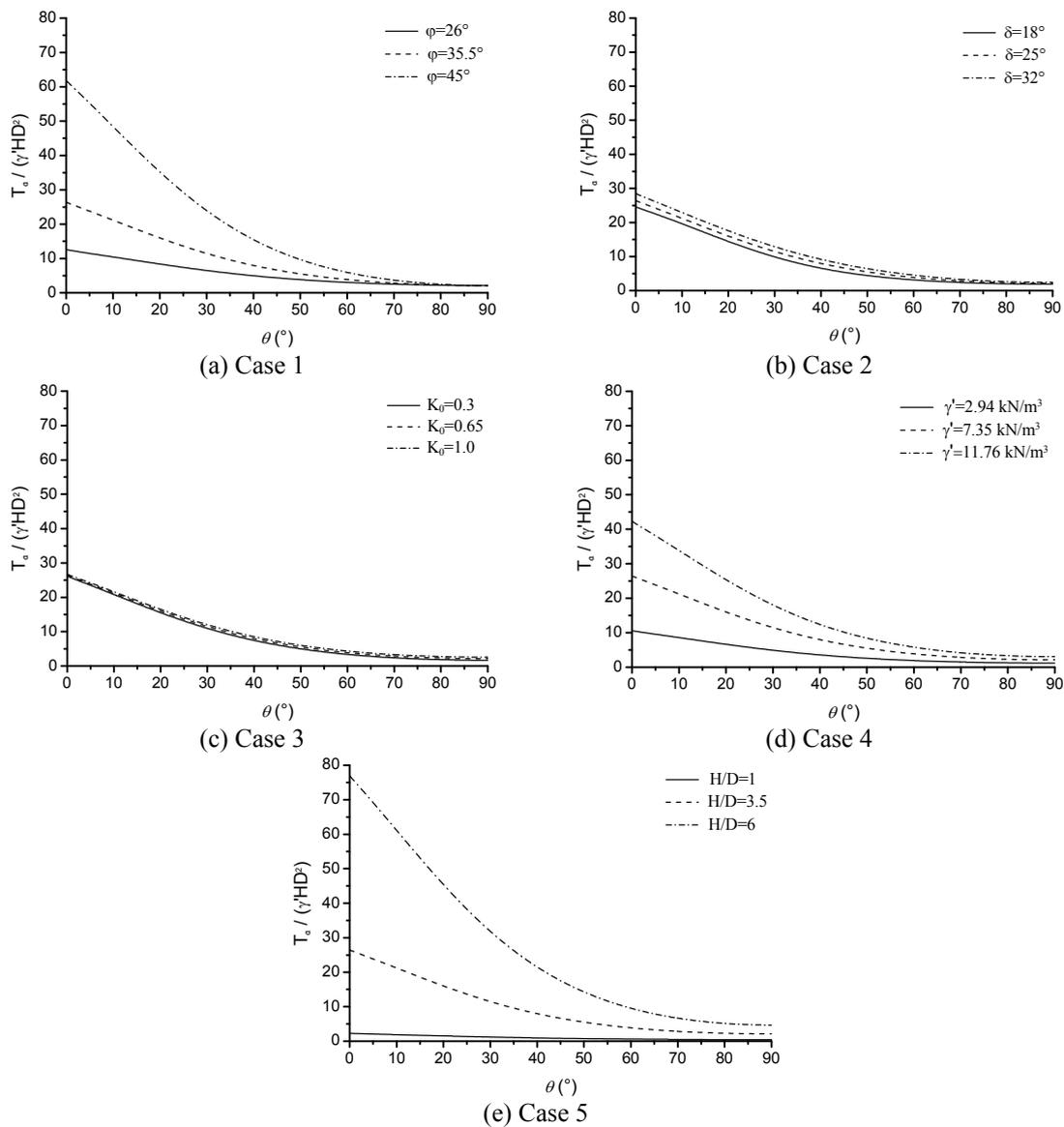
Fig. 4 Effects of different parameters on the ultimate pullout capacity of suction anchors
