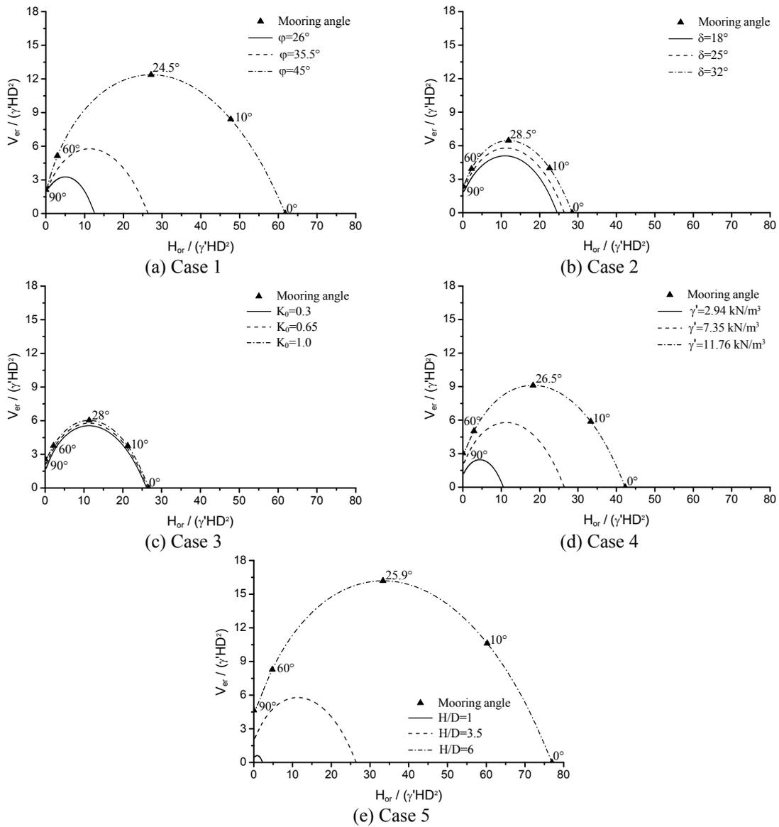
Fig. 5 Effects of different parameters on the relation between horizontal and vertical pullout capacities of suction anchors
